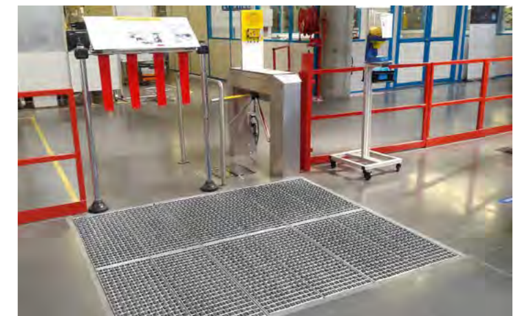
Cleaning of soles and rollers by ProfilGate® st55 go in front of the ESD-area
