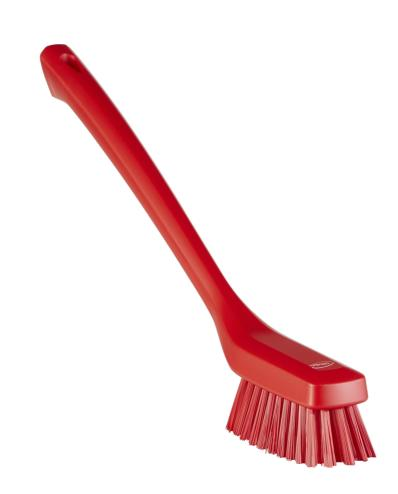
Easily clean small spaces with this 46 mm wide narrow-headed brush. The bristles are angled to facilitate easy cleaning of corners, the grip is designed for extra stability and the entire brush is color-coded to support HACCP principles.
