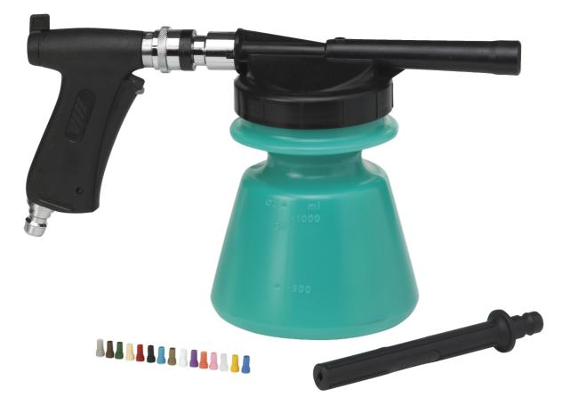
Clean sanitary and small processing areas, applying foam at normal water pressure. Ensures consistently correct dosage (0.4–10%). Colour-coding facilitates chemical identification. Safeone (9340) is recommended for protection against chemical reflux in potable water supplies and is approved according to EN 1717 - substance class 3.
