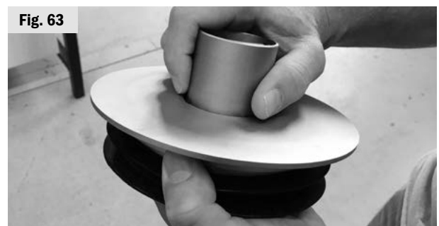
4. In order to change the fill level, remove the overflow plug from the drain and turn the pipe sticking out against the seal regulator. Unscrew the pipe counter-clockwise to increase the fill level. Screw in the pipe clockwise to lower the fill level. Test a new setting and make sure that the tray does not overflow.
