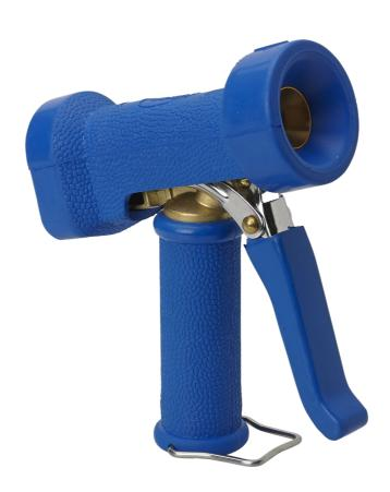
The Heavy Duty Water Gun is suitable for cleaning floors and machinery, and for rinsing off work surfaces and walls after chemical foaming. Determine the jet pattern by squeezing the rubber insulated trigger. Adjust the water jet with a screw at the end of the gun. An arrow on the gun shows the water spray direction. Use 0712 1/2" or 0715 3/4" hose nipples, which can be screwed into the bottom of the gun. You need one of these nipples to connect a hose to the gun.
