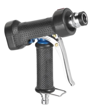
This is a replacement piece for the Foaming Set (9303x). A rubber coating ensures a good grip during use, even in wet conditions. The foaming gun has a 1/2" nozzle that can connect to a 1/2" Q coupling.
