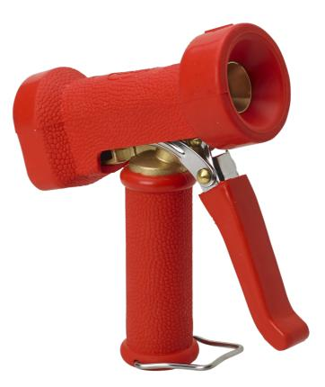
The Heavy Duty Water Gun is suitable for cleaning floors and machinery, and for rinsing off work surfaces and walls after chemical foaming. Determine the jet pattern by squeezing the rubber insulated trigger. Adjust the water jet with a screw at the end of the gun. An arrow on the gun shows the water spray direction. Use 0712 1/2" or 0715 3/4" hose nipples, which can be screwed into the bottom of the gun. You need one of these nipples to connect a hose to the gun.
