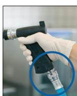
7. The hose with ½" quick-coupling (item no. 0702) is connected to nipple on the water gun.
