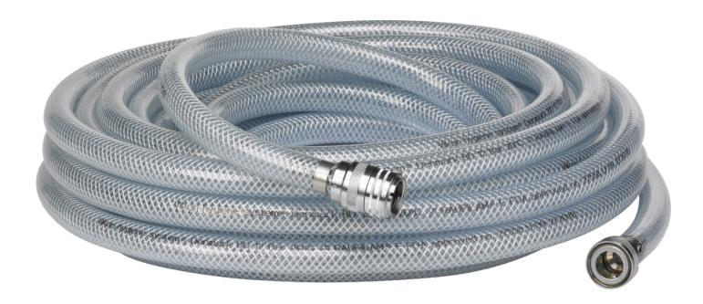
For cold water cleaning up to  $40^{\circ}$  C, that 1/2" ready-to-use hose features a 1/2" clutch housing at both ends. Water tap nipple provided for 1/2", 3/4" and M22x1 screw thread types.
