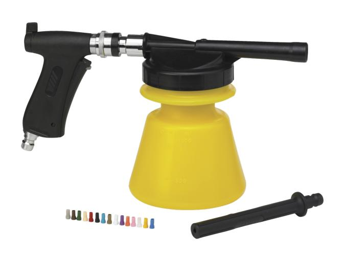
Clean sanitary and small processing areas, applying foam at normal water pressure. Ensures consistently correct dosage (0.4–10%). Colour-coding facilitates chemical identification. Safeone (9340) is recommended for protection against chemical reflux in potable water supplies and is approved according to EN 1717 - substance class 3.
