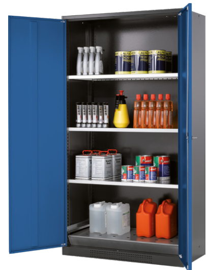
Cabinet for chemicals CS-CLASSIC model CS.195.105 body colour anthracite grey (RAL 7016), with wing doors in gentian blue (RAL 5010), interior equipment with 3 x shelf, 1 x perforated insert, 1 x bottom collecting sump (sheet steel galvanised) Order No. 30495-047-30508
